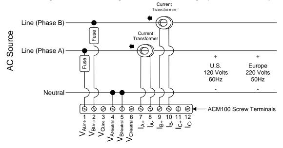
Figure 4 – Single-Phase (Dual Line) Connection Diagram
